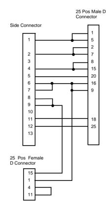
Figure 3-16 Wiring of the Connectors
