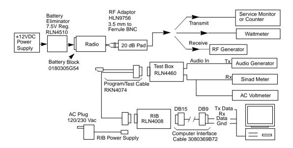
Figure 5-1 Radio Tuning Test Equipment Setup
