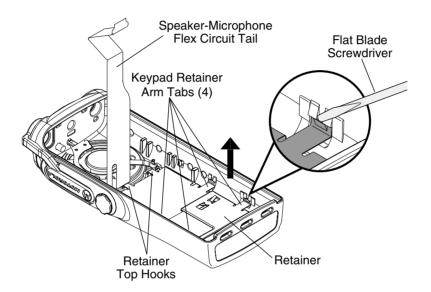
Figure 3-6 Remove Retainer
