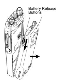
Figure 3-1 Battery Removal
