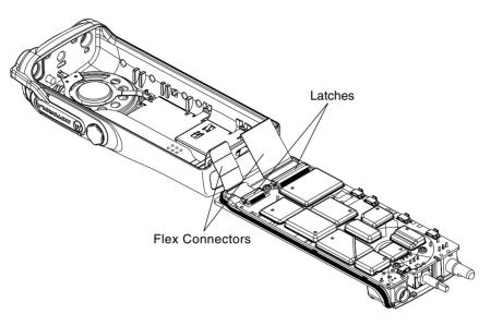
Figure 3-4 Unlatch Flex Connectors
