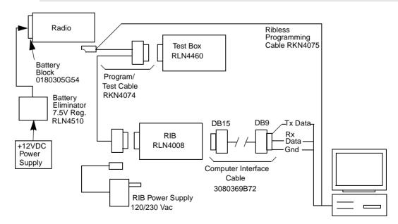
Figure 5-2 CPS Programming Setup
