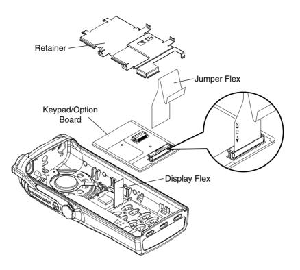
Figure 3-12 Changing the Keypad/Option Board
