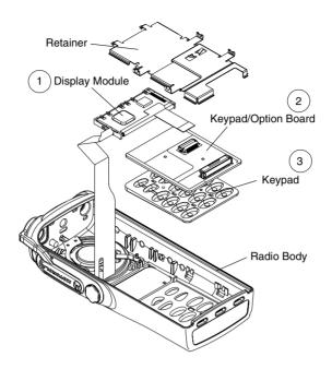
Figure 3-7 Removing the Keypad Retainer and Other Boards from the Radio Body
