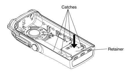
Figure 3-10 Lock retainer catches to the radio's body
