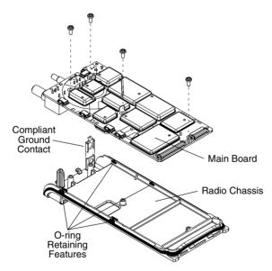
Figure 3-5 Remove Main Board from Chassis
