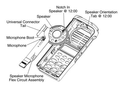
Figure 3-8 Removal Speaker-Microphone Assembly
