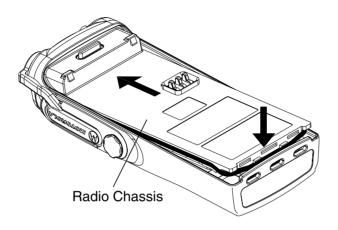
Figure 3-11 Fastening the Chassis
